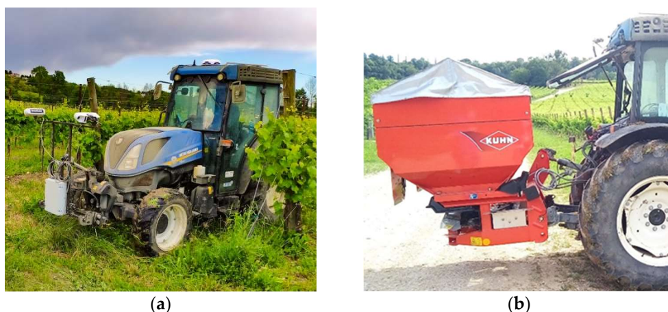
Figure 3. Working configuration during the fertilizer application: (a) The Greenseeker sensor system; (b) The fertilizer spreader.
